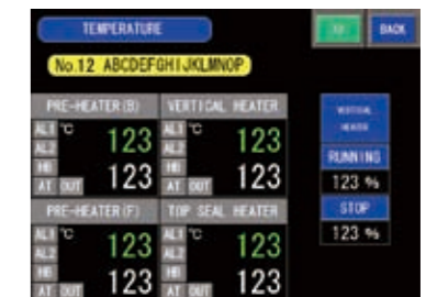
Temperature control screen
